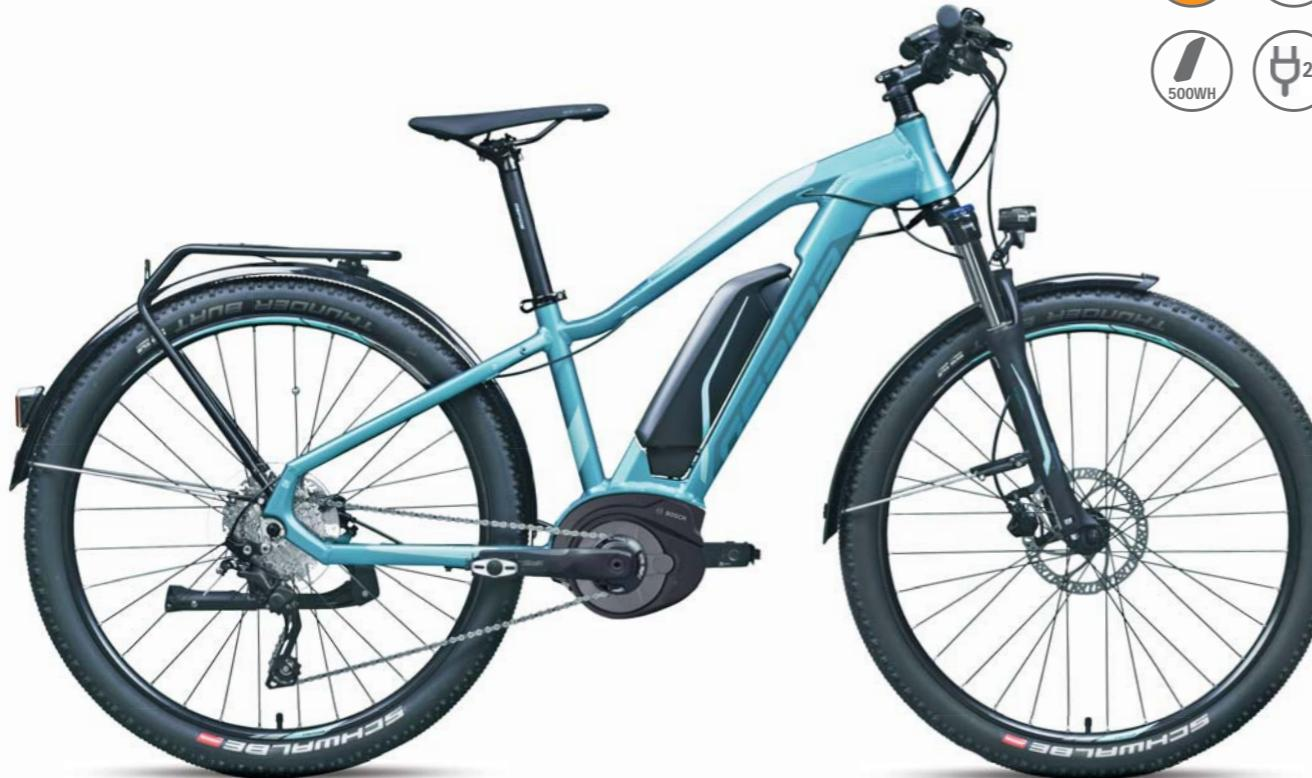
△ FRAME GEPIDA HYDROFORMING - 6061 ALLOY
