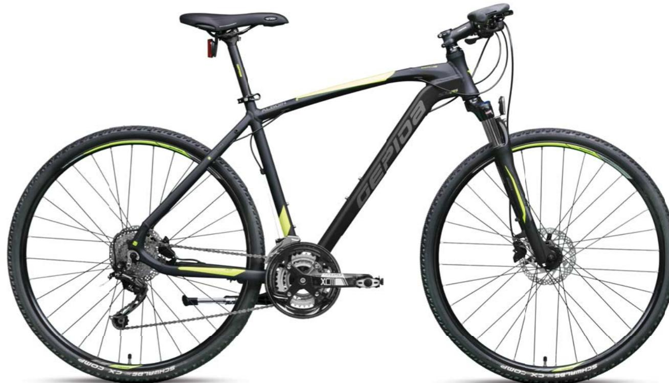
△ FRAME GEPIDA HYDROFORMING - 6061 ALLOY
