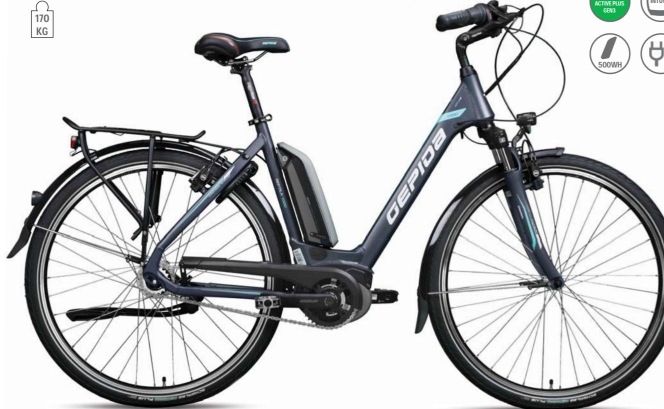
△ FRAME GEPIDA HYDROFORMING - 6061 ALLOY
