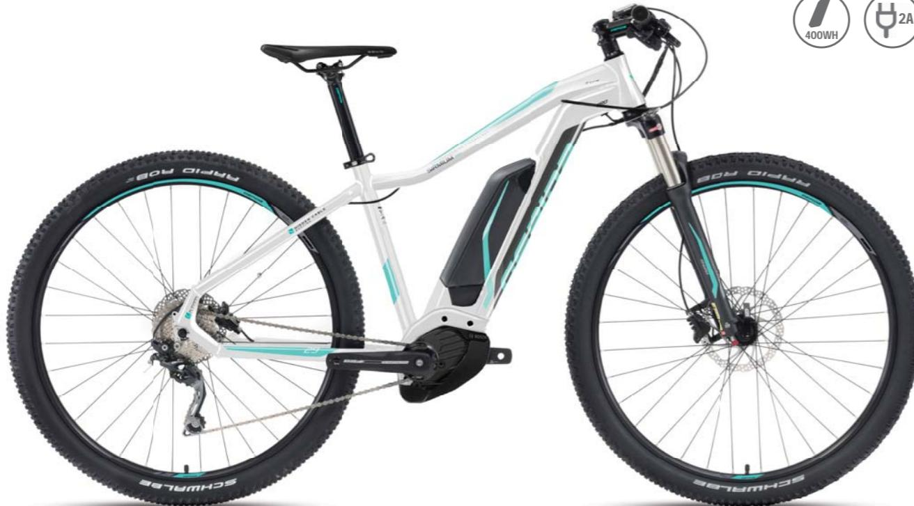
△ FRAME GEPIDA HYDROFORMING - 6061 ALLOY
