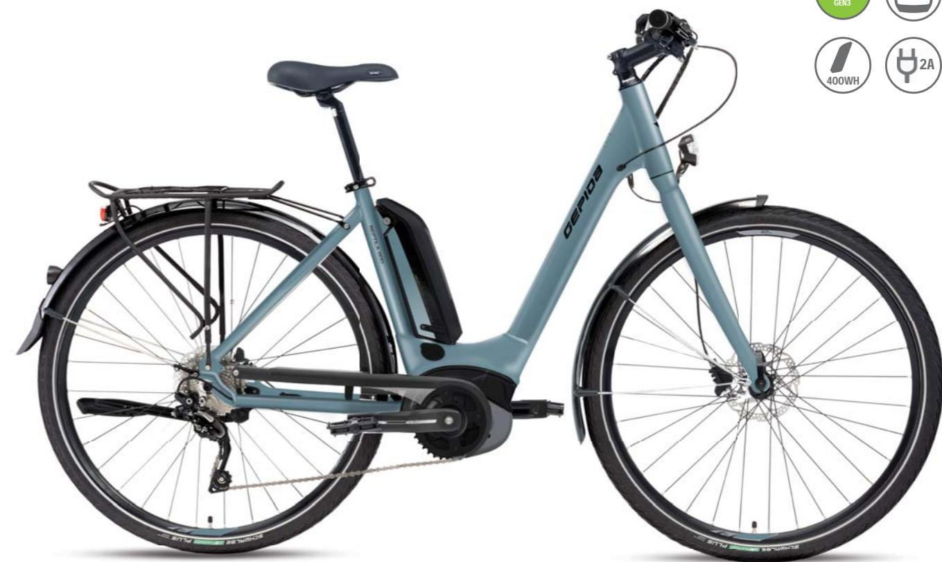
☐ FRAME GEPIDA HYDROFORMING - 6061 ALLOY
