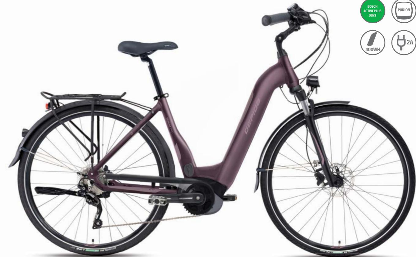
△ FRAME GEPIDA HYDROFORMING - 6061 ALLOY
