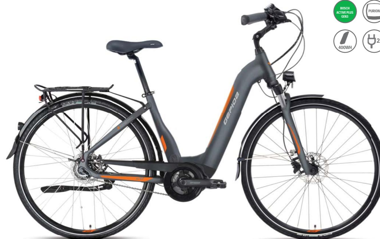
△ FRAME GEPIDA HYDROFORMING - 6061 ALLOY
