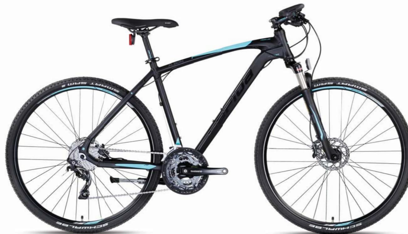
△ FRAME GEPIDA HYDROFORMING - 6061 ALLOY
