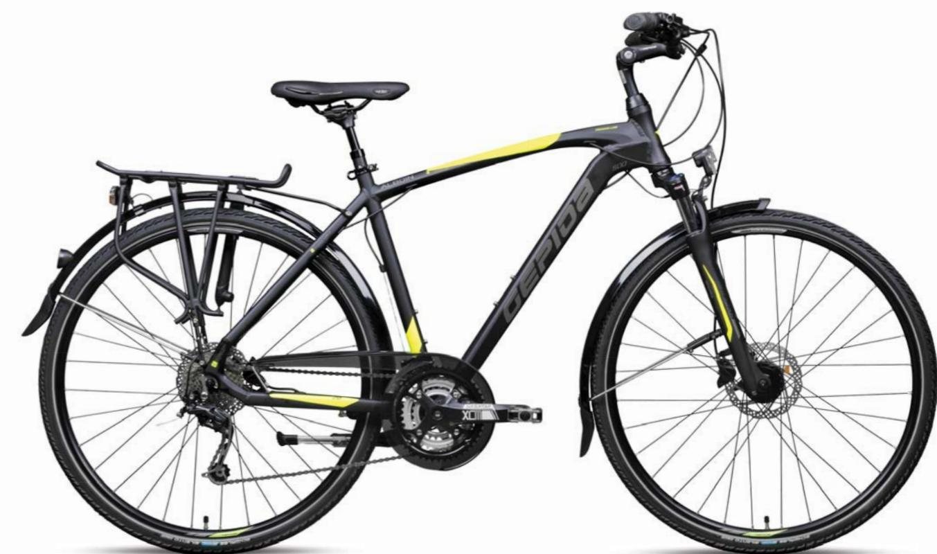
△ FRAME GEPIDA HYDROFORMING - 6061 ALLOY
