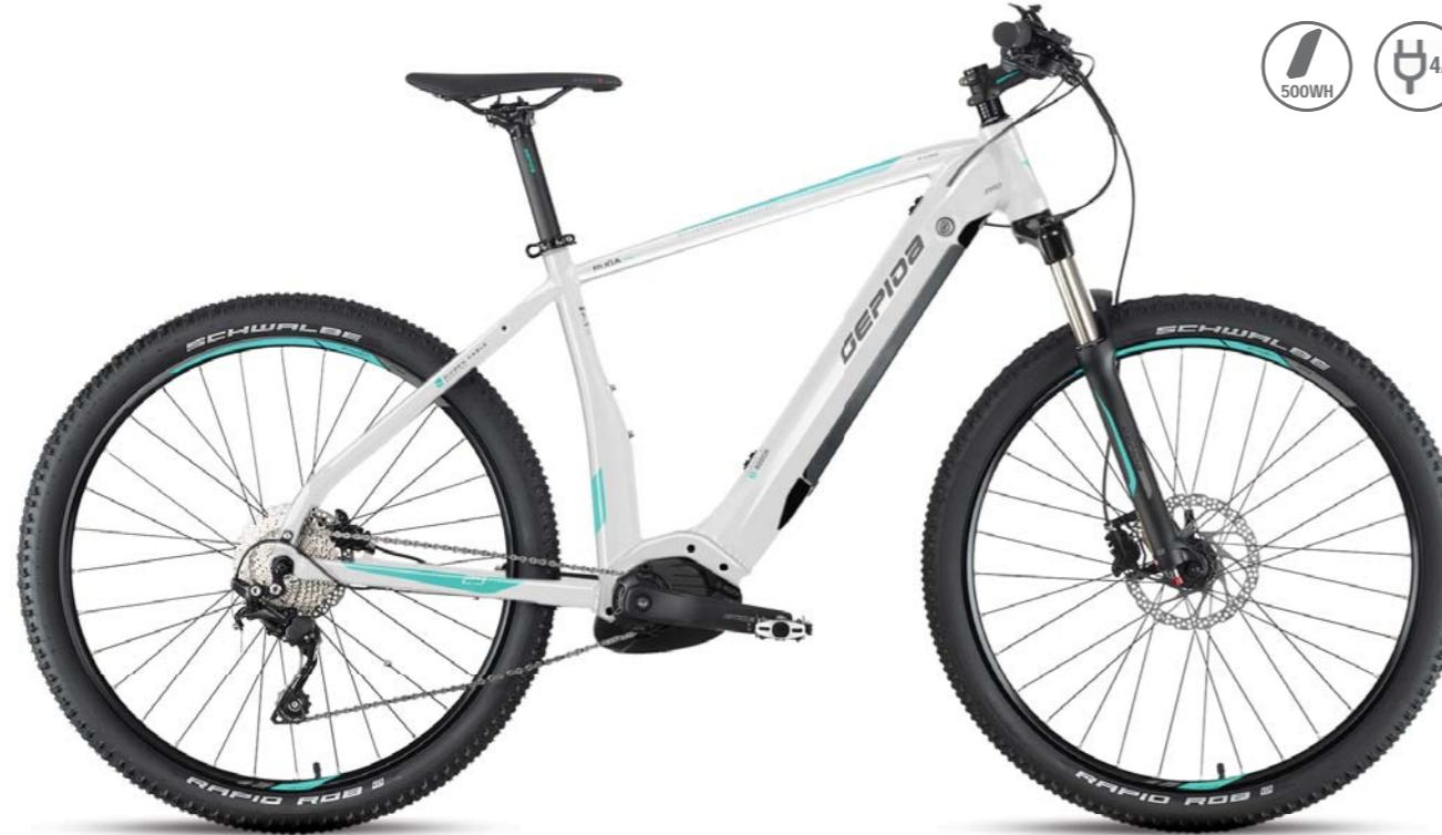
△ FRAME GEPIDA HYDROFORMING - 6061 ALLOY
