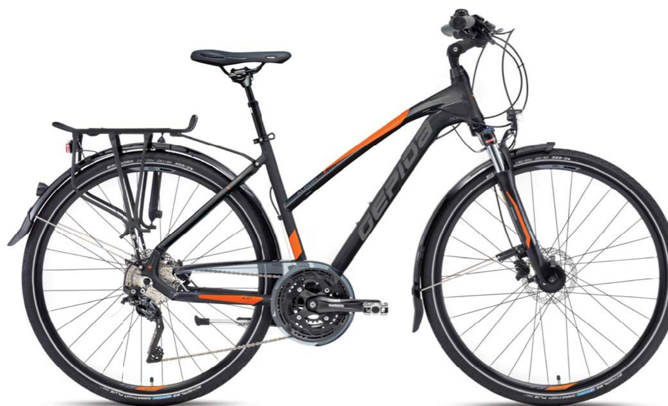
△ FRAME GEPIDA HYDROFORMING - 6061 ALLOY
